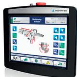
The main features of the HBG 0811 handheld panel from **Sigmathek** is its light weight of 950 g that enables hours of fatigue-free operation, plus an
